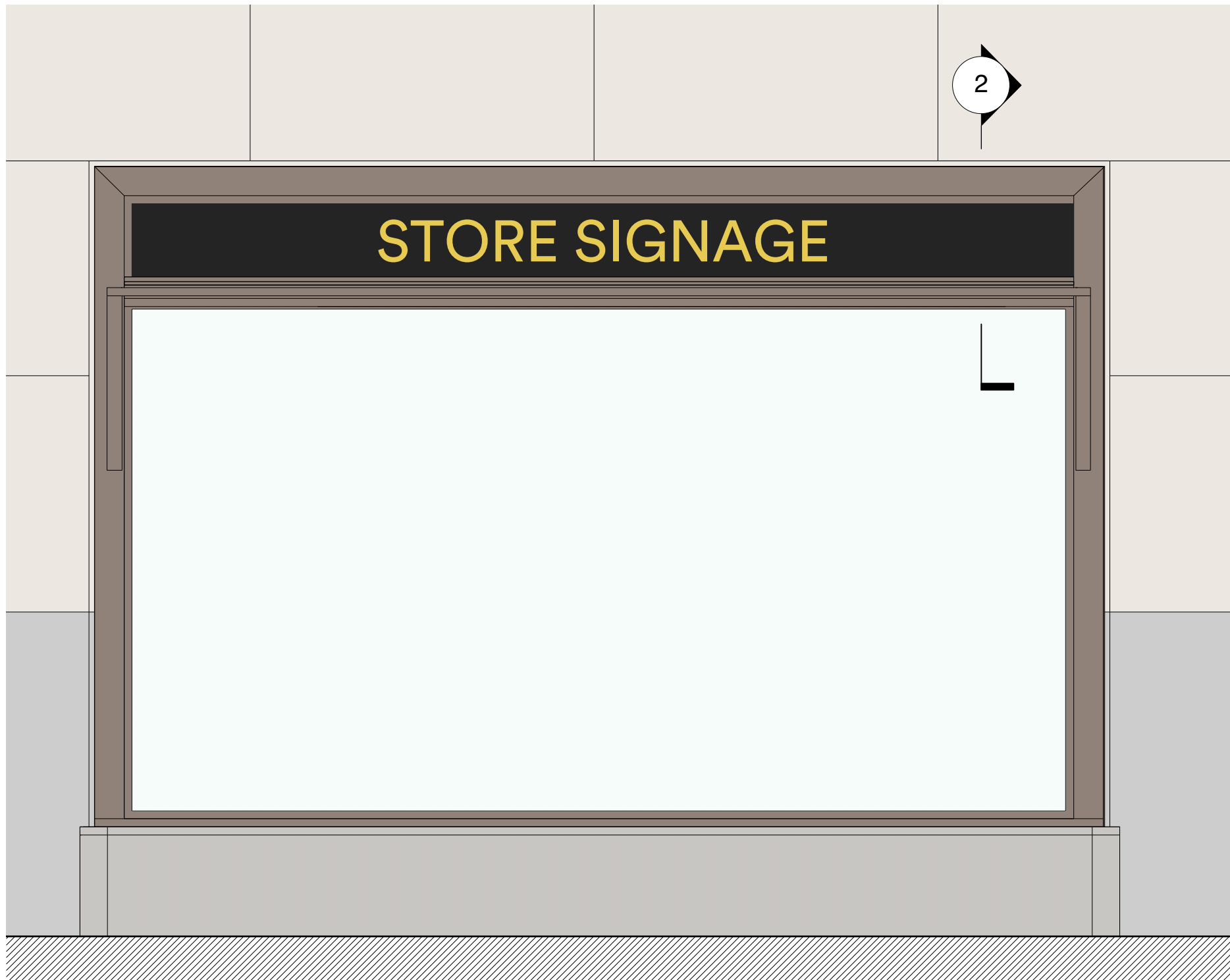
1 EDGE LIT & FACE LIT BRONZE LETTER - ELEVATION SCALE: 1/2" = 1'-0"
