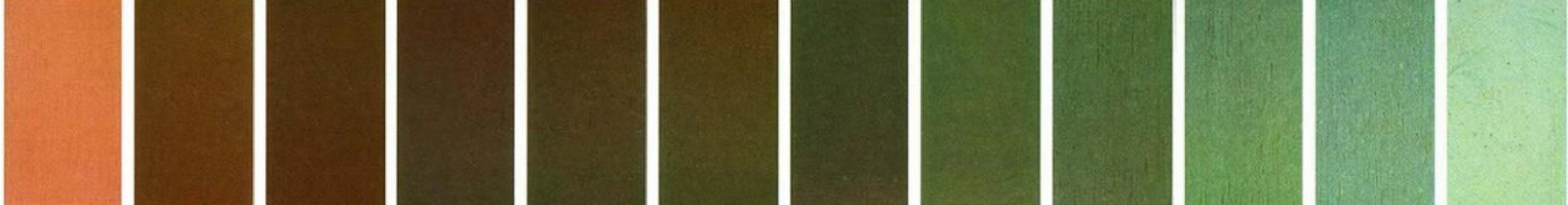
UNEXPOSED COPPER 4 MONTHS 8 MONTHS 1 YEAR 2 YEARS 3 YEARS 4 YEARS 5 YEARS 7 YEARS 10 YEARS 15 YEARS 20+ YEARS
