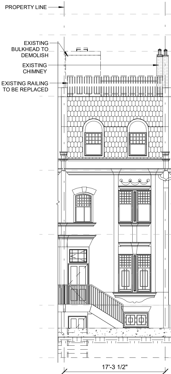
EXISTING FRONT ELEVATION
