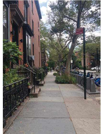
A new bluestone sidewalk and curb in the Cobble Hill Historic District matches the adjacent historic bluestone pavers in dimension, color, and paving pattern.
