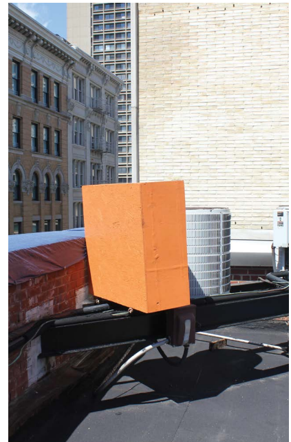
The orange box is a physical mock-up of a proposed rooftop HVAC unit. Staff may require such a mock-up to determine an installation's potential visibility from public thoroughfares.
