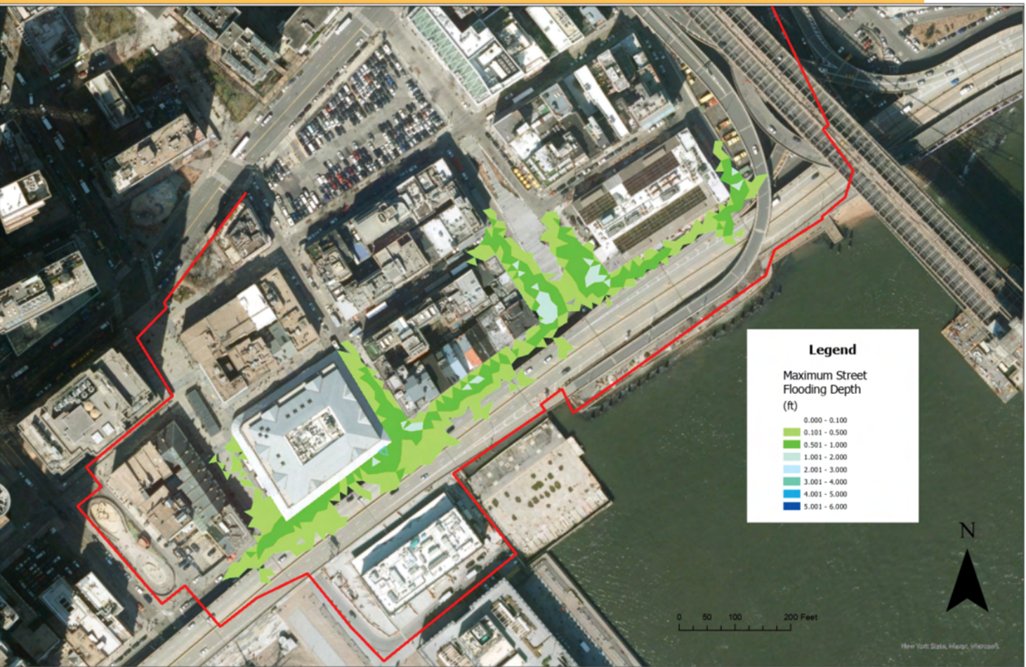
WITH SEWER ISOLATION & SUPPLEMENTAL PUMPING NEAR REGULATOR
