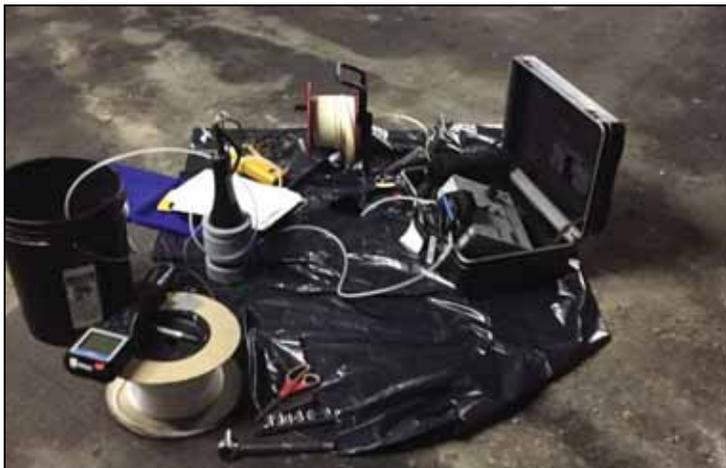
**Photograph 7.** Low-flow groundwater sampling.
