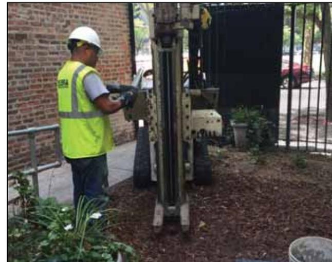
**Photograph 8.** Limited access retrofitted track-mounted direct-push probe unit advancing soil boring in the garden area of 145-149 West 108<sup>th</sup> Street.
