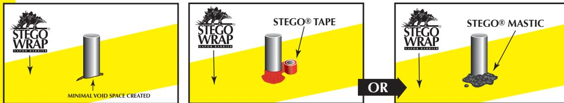
**STEGO WRAP PIPE PENETRATION REPAIR DETAIL:**
