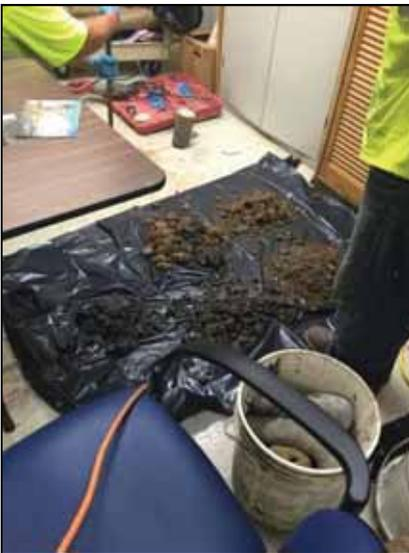
**Photograph 3.** Soil from hand auguring laid out on plastic prior to sampling in 145-149 West 108<sup>th</sup> Street basement.
