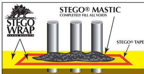
**MULTIPLE PIPE PENETRATION SEALING:**
