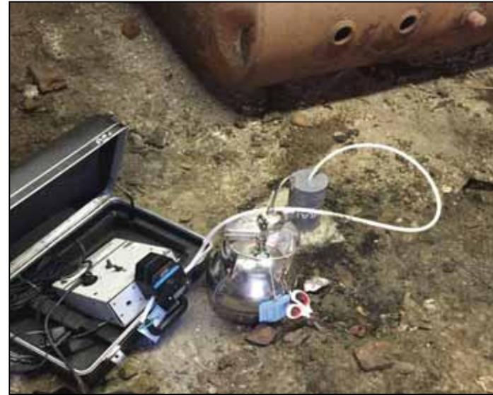
**Photograph 2.** Purging soil vapor point prior to sampling in the partial basement of 103-107 West 108<sup>th</sup> Street.
