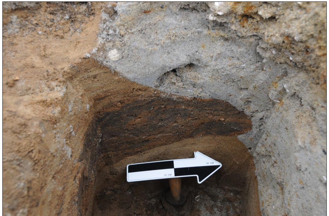
Facing west showing west wall of Test Pit 2.1 at a depth of 12 feet below ground surface in Trench 2. Note mixed sandy fills overlying subsoils
