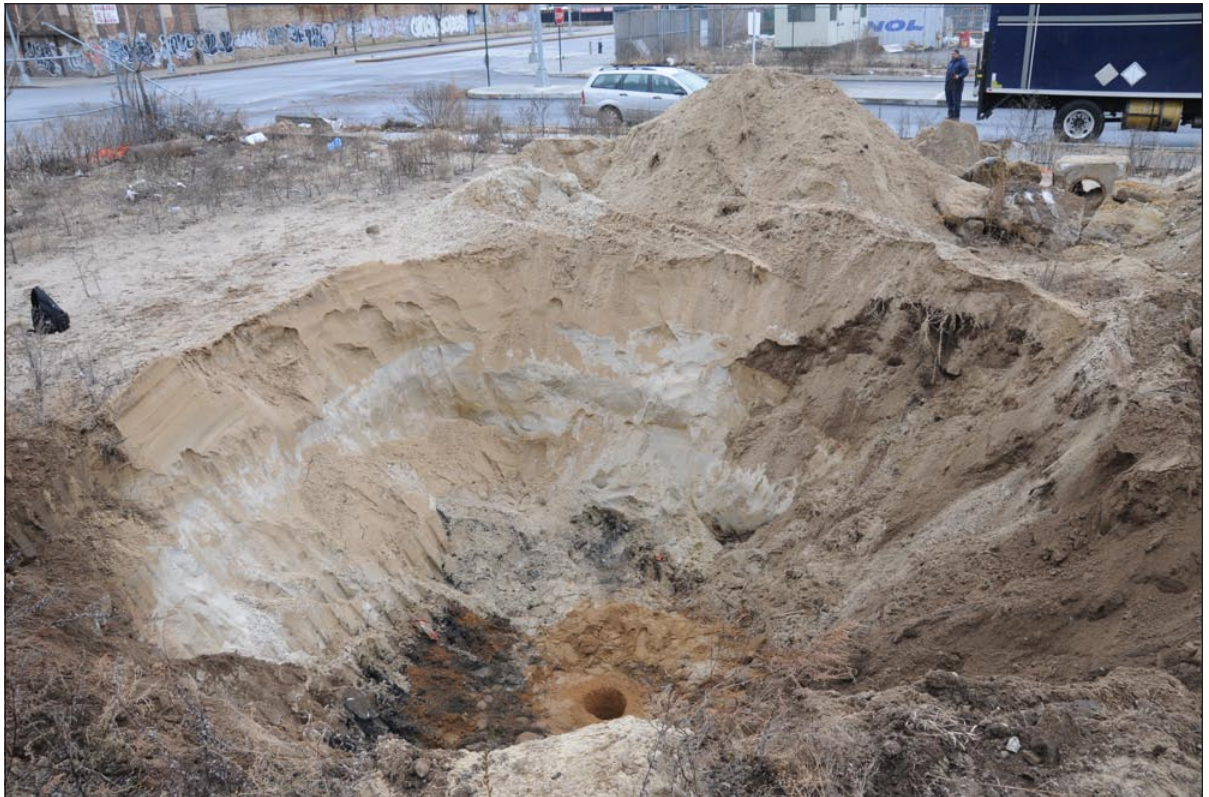
Facing east showing completed Trench 1 with Test Pit 1.1 located at its bottom and Elton Street in the background. Note 10 feet of loose sandy fill overlying natural subsoils
