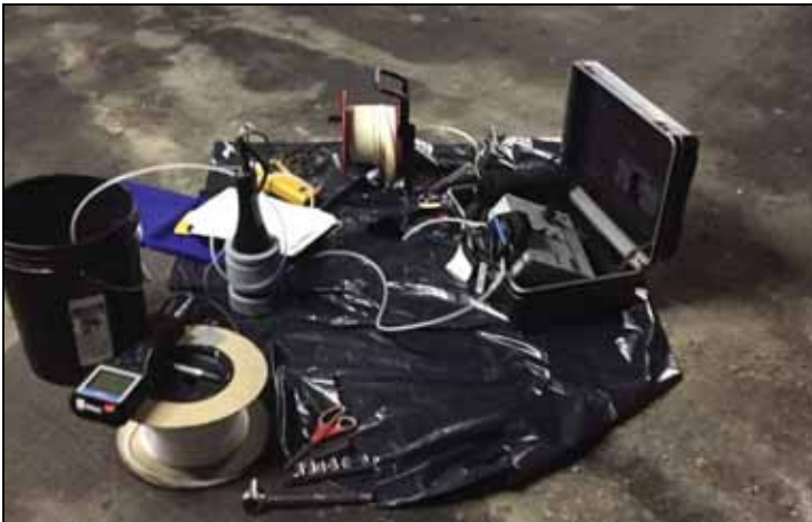
Photograph 7. Low-flow groundwater sampling.
