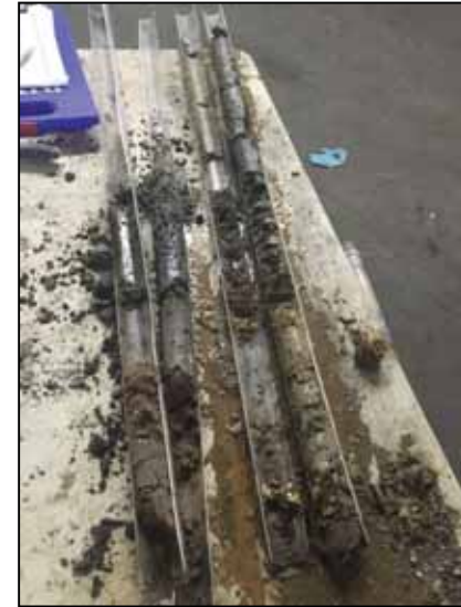
Photograph 6. Soil cores showing borehole contents after collecting soil samples.
