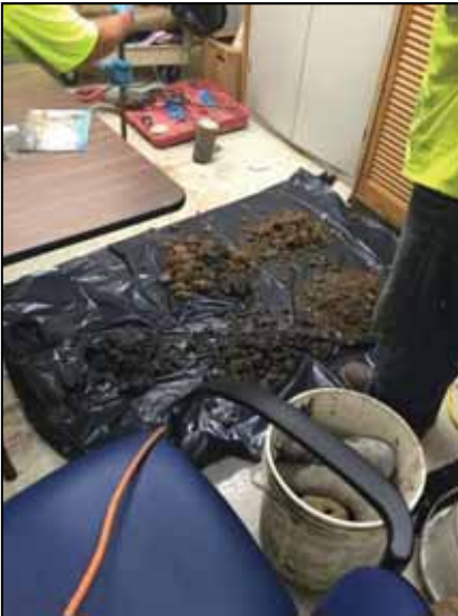
Photograph 3. Soil from hand auguring laid out on plastic prior to sampling in 145-149 West 108 th Street basement.
