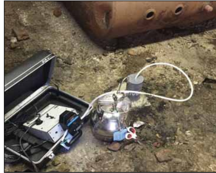
Photograph 2. Purging soil vapor point prior to sampling in the partial basement of 103-107 West 108 th Street.
