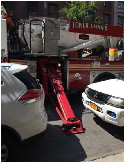
Photo 3 - Outrigger between Parked Cars
