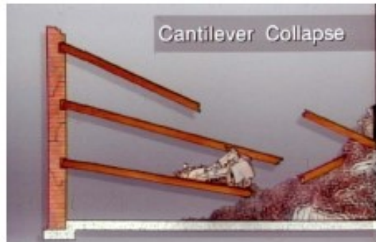
Cantilever Collapse (Unsupported Lean-To) Greatest Potential For Secondary Collapse
