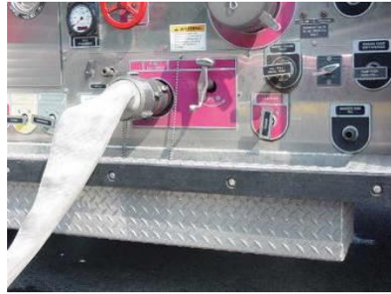
3 1/2" hose into operating pumper
