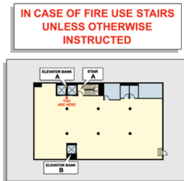
Elevator landing signs - separated
