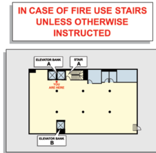
Elevator landing signs - separated
