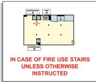
Elevator landing sign
