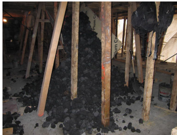
Unsafe (unorderly) stored coke
