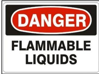
Warning signs must be made of durable material. Signs warning of the hazard of flammable liquids must have red, black or white lettering on a contrasting background and must read: DANGER—FLAMMABLE LIQUIDS.
