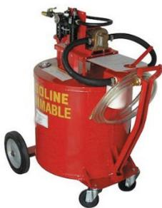
Defueling equipment must be **listed** for defueling purposes and its capacity cannot exceed **65gal.**
