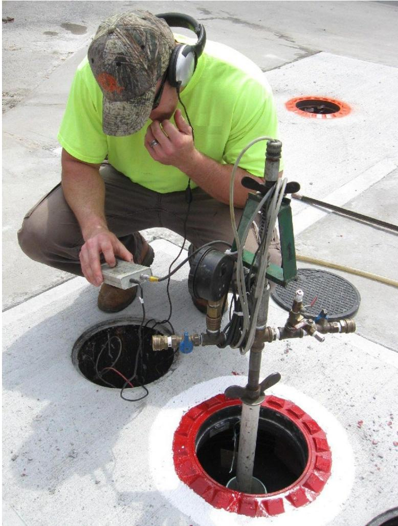
**An approved precision testing system for tanks and piping (vacuum test).**
