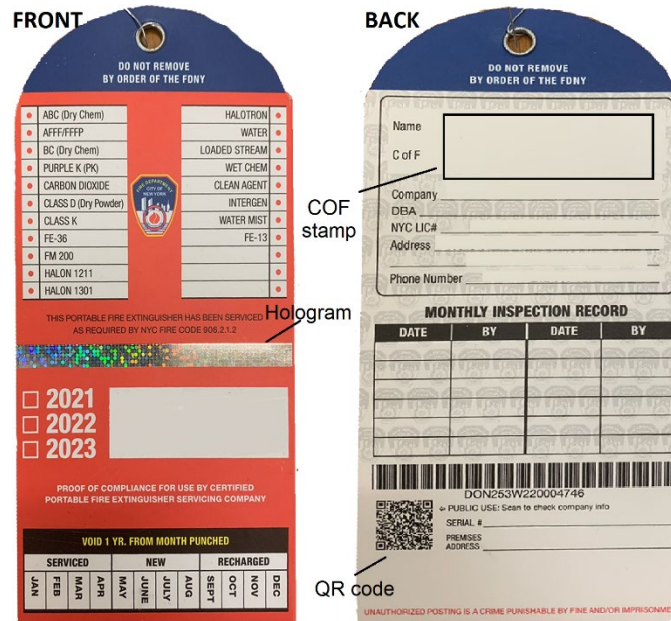
PFE tag (This tag was released for 2021-2023) Tag colors and year will change every few years for security purposes.
