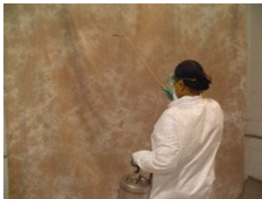
Examples of fabric being sprayed with a flame retardant chemical
