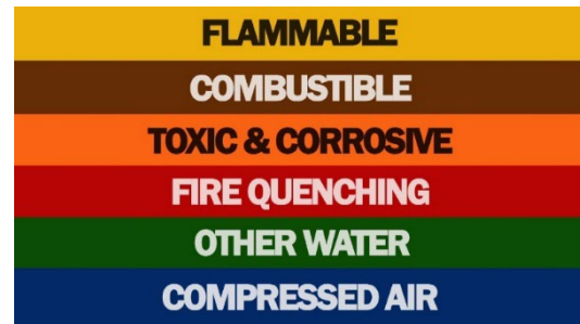
ASME A13.1 Piping label color chart
