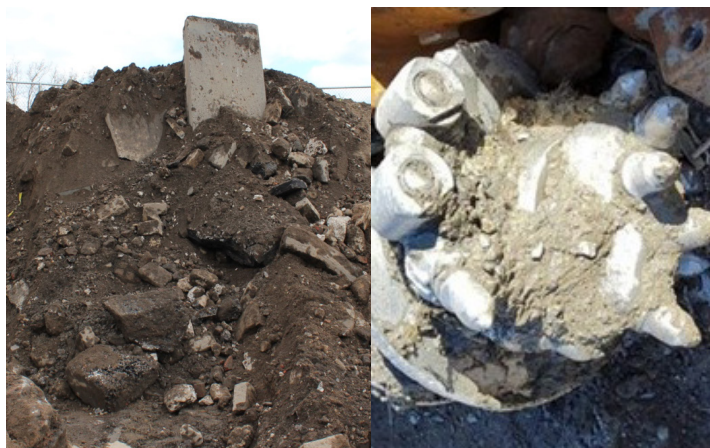
Historic urban fill and drill bit teeth damaged by obstructions, November 2025
