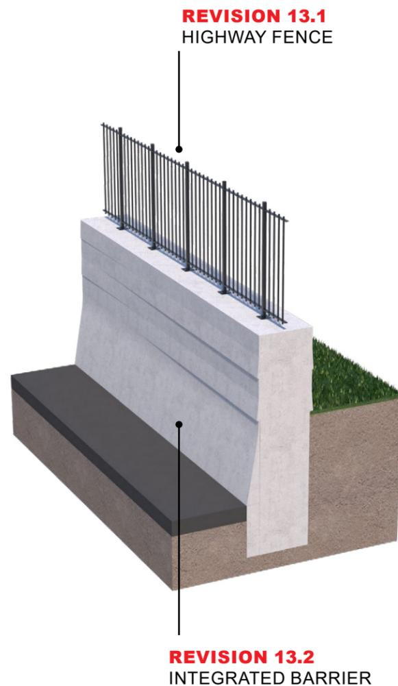
INTEGRATED FLOOD/RETAINING WALL AND TRAFFIC BARRIER
