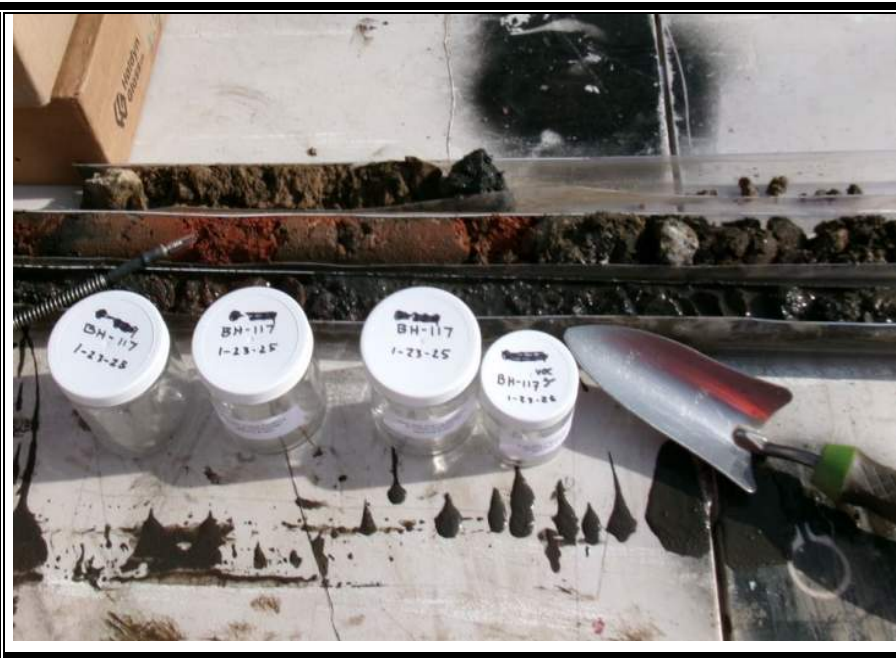
Soil boring BH-117, (haz location), collected 1/23/25
