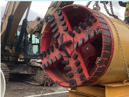
Microtunneling machine on site - December 2024
