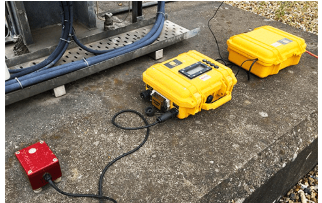
Example of Vibration Monitor
