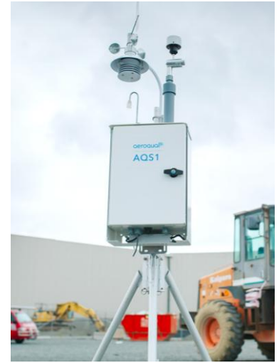
Example of Air Quality Monitor
