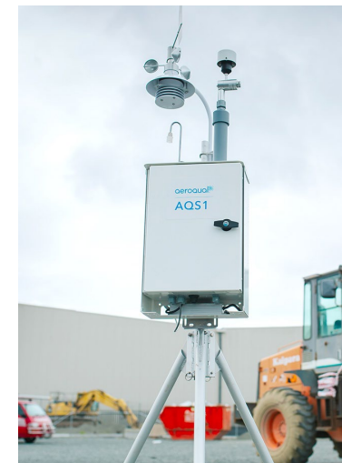
Example of Air Quality Monitor
