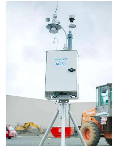
Example of Air Quality Monitor
