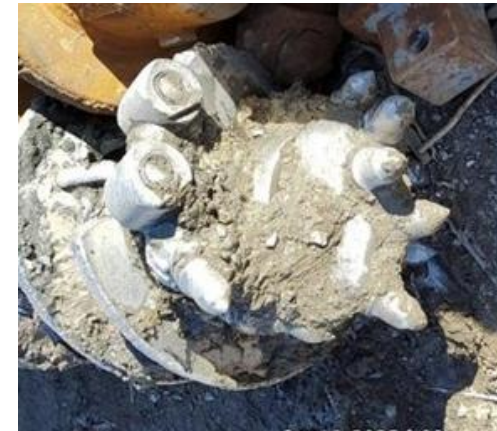
Drill bit teeth damaged by obstructions
