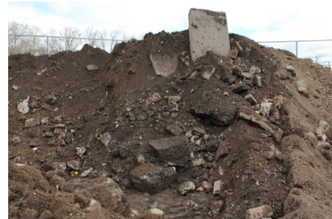
Excavated historic urban fill material, including masonry bricks, coarse rocks, timber bulkheads
