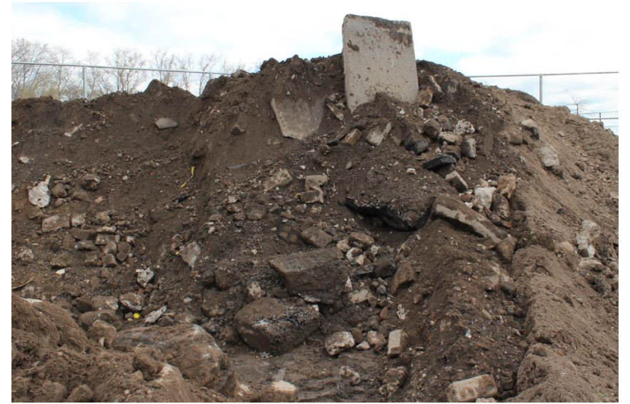
Excavated historic urban fill material, including masonry bricks, coarse rocks, timber bulkheads
