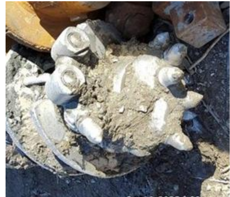
Drill bit teeth damaged by obstructions
