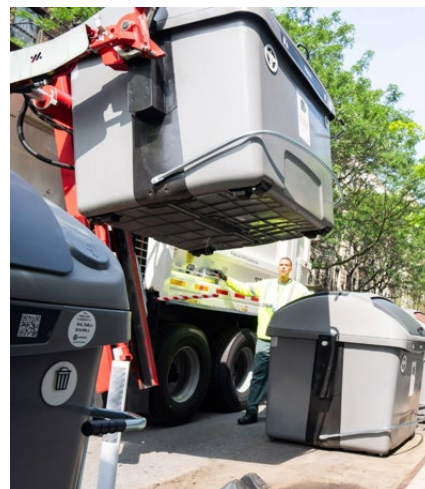
Figure 6: Arms of ASL trucks grab, lift, and empty containers
