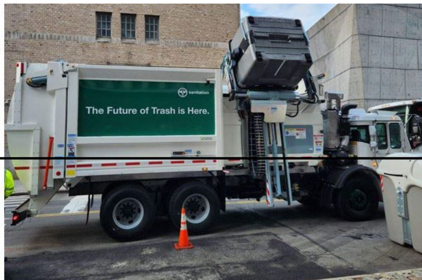
Figure 1-5. Automated Side Loader (ASL) Collection Vehicle
