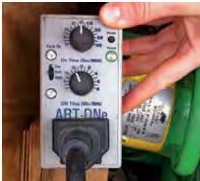
Timer used to control how often and for what duration the fan is on.
