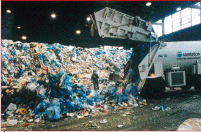
DOS workers tip blue bags full of metal, glass, and plastic recyclables at a material recovery facility (MRF) for processing by private contractors.
