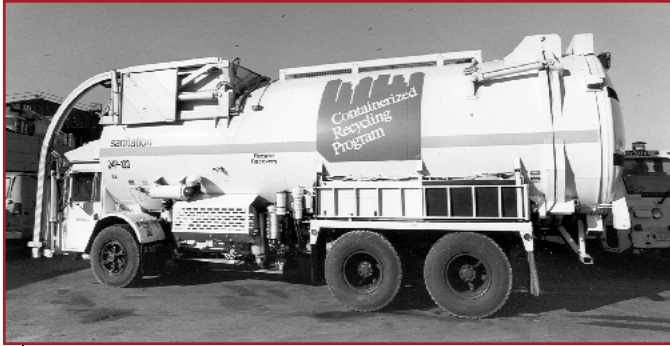
This containerized packer truck is able to collect metal dumpsters full of recyclables.
