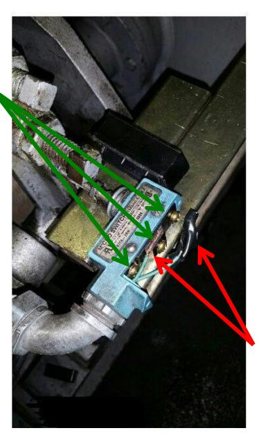
but instead, the wires were not connected to the screws, and both stripped wire tips were covered in black electrical tape.
