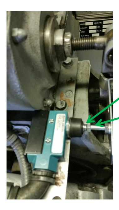
To function, the brake monitor microswitch must make contact with the linkage bolt.
