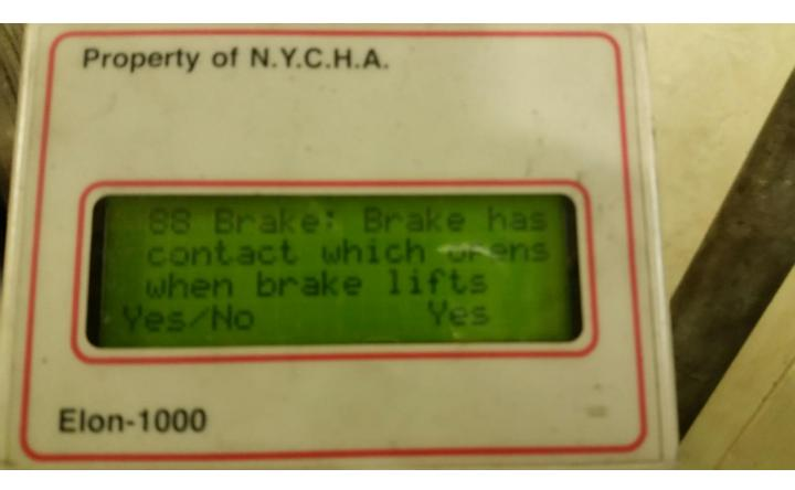
**Tricon Handheld Device, Setup Parameter 88**
