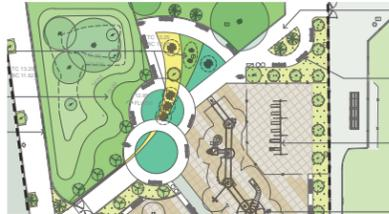
A complete reconstruction, with new grading and bioswales, will increase site permeability and reduce stormwater runoff for this park sited within the 100-year floodplain. A bermed lawn area with shade trees buffers the spray play area and creates a more inviting park edge along the street. New play spaces accommodate children of all abilities, and shaded, family-friendly picnic areas and benches will be added within the park and along its perimeter.
