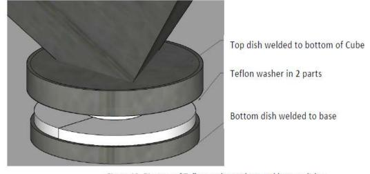
Figure 10. Diagram of Teflon washer and top and bottom dishes
