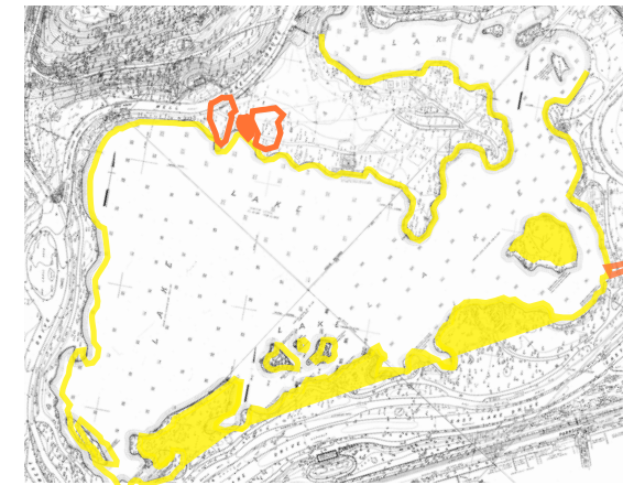
1937 Plan Plan shows consolidation of islands, filling of shallow areas in the lake, and retaining walls along the shoreline.
