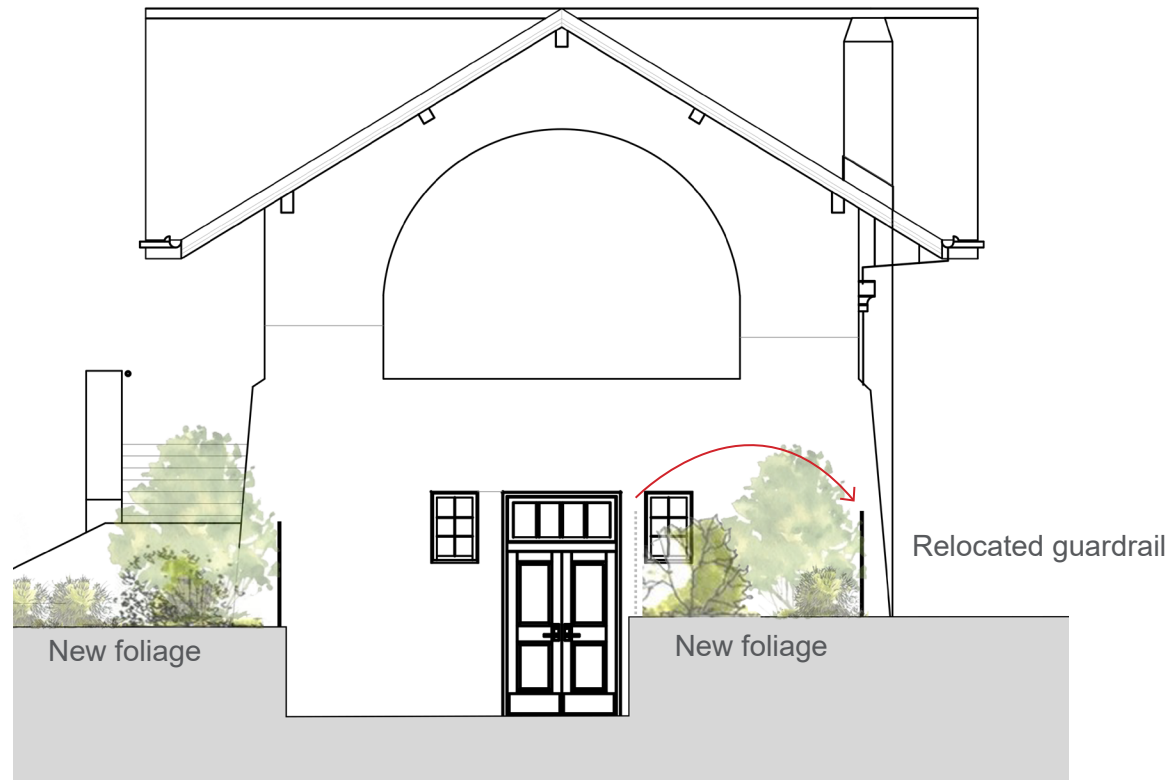
PAVILION EAST FACADE - AREAS WHERE PEOPLE CAN ACCESS THE BUILDING. SECURITY MEASURES NEEDED
