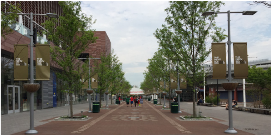
TYPE Pole Lights LOCATION Pedestrian walkways and drop off areas PROPERTIES Selux (match existing) post mounted, LED double arm fixture, 16’ High
