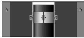
Sign Section: Cap Detail with Pole Installation
