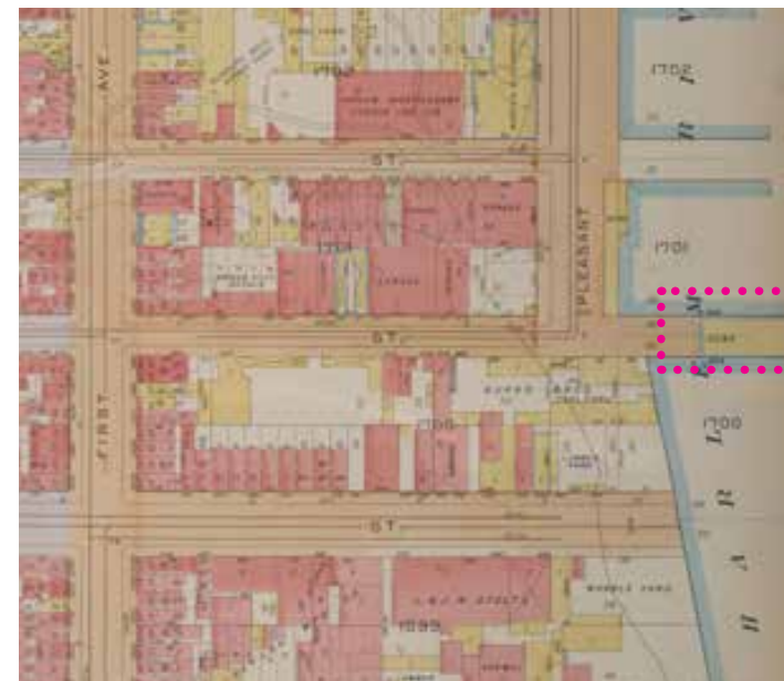
1923 107th Street pier "dump" indicated as a wood frame structure with metal cladding; large coal, marble and lumber yards seen at water's edge
