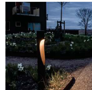
● ELT03: Bollard LED Material: Aluminum Size: 31.5" tall Color: 'Corten' Finish: Powder coated Manufacturer: Louis Poulsen Product Line: Flindt
