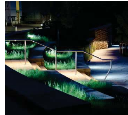
ELT01: Handrail Light Material: Aluminium Manufacturer: Klik USA Product Line: LEDpod40 Finish: Clear Anodized
