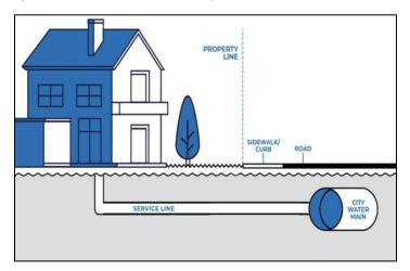
In the past, many service lines for smaller buildings, mainly 1-4 family homes, were made of lead. When water sits in a lead pipe, particularly for several hours, the lead can leach into the water.
