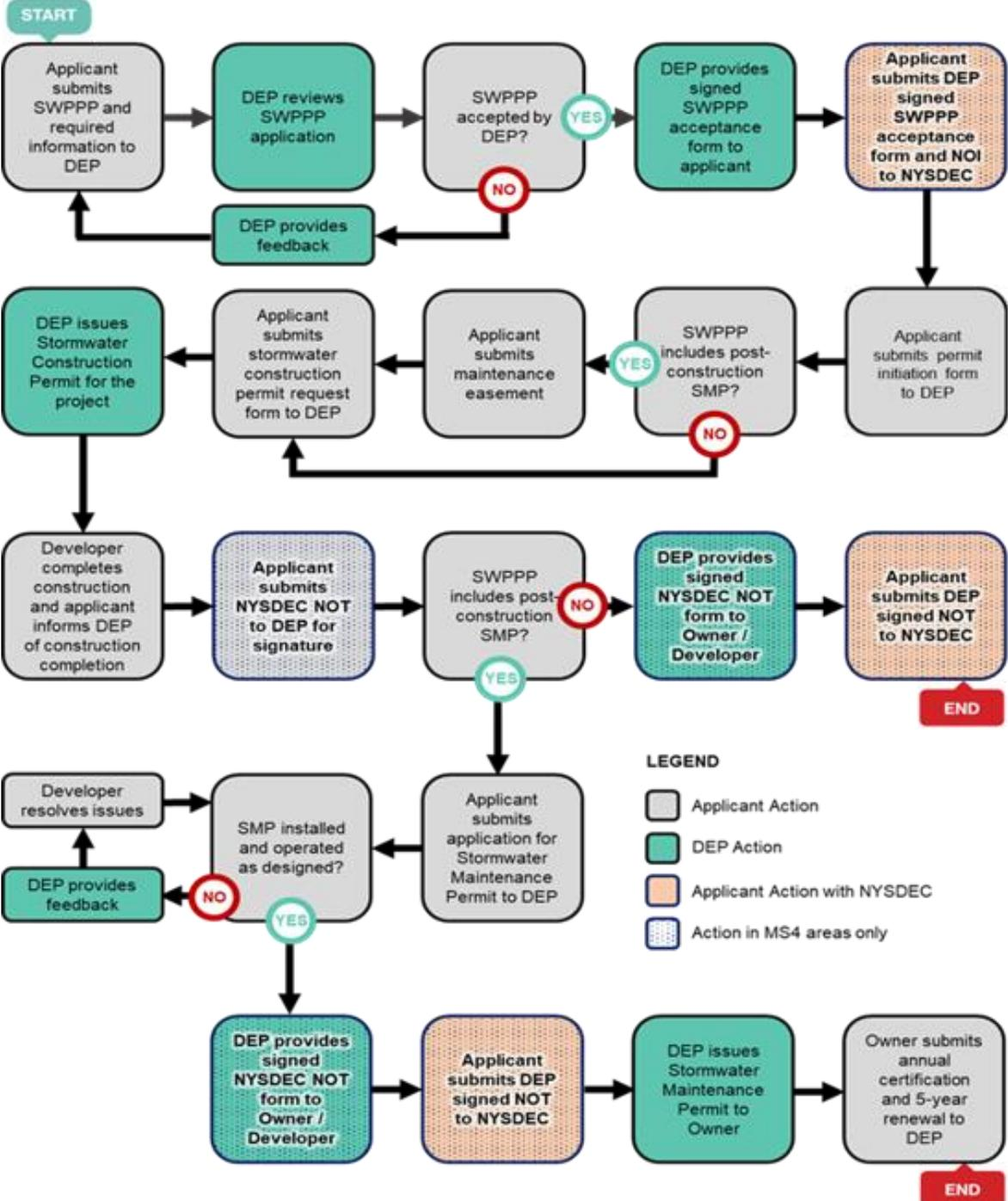
Flow diagram #5: detailed process for stormwater construction permits
