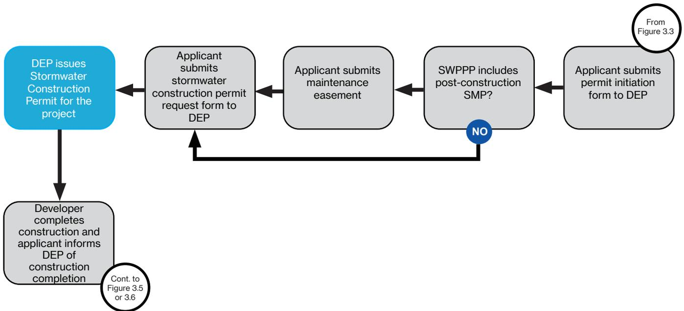
**Figure 3.5.** SWPPP Does Not Include Post-Construction SMP Decision Point.
