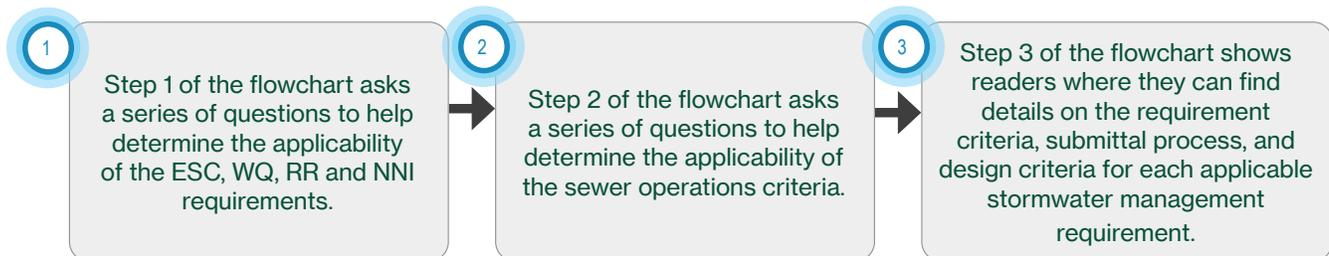
**Figure 2.3.** Flowchart to help determine applicable stormwater management requirements and procedures.
