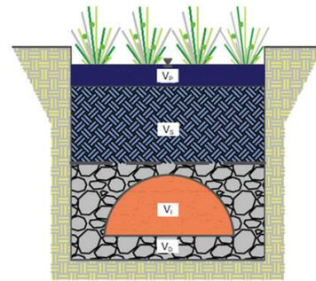
During the design process, designers should also consider any other factors which may impact the size of the overall practice or specific elements. For example, the elevation of the overflow device will govern the top of the active storage zone, which may impact the depth of drainage media that may be counted towards SMP storage volume.
