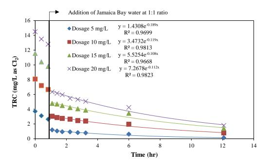
Figure 2. Spring Creek chlorine degradation at varying chlorine dosages.
