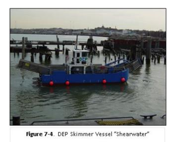
DEP currently has two self-propelled skimmer vessels (Aquarius Systems Custom Model HSTH235 - High Speed Trash Hunter) and one old vintage skimmer vessel which must be towed. DEP relinquished 1 vessel in April 2019 and is currently procuring a new vessel.
