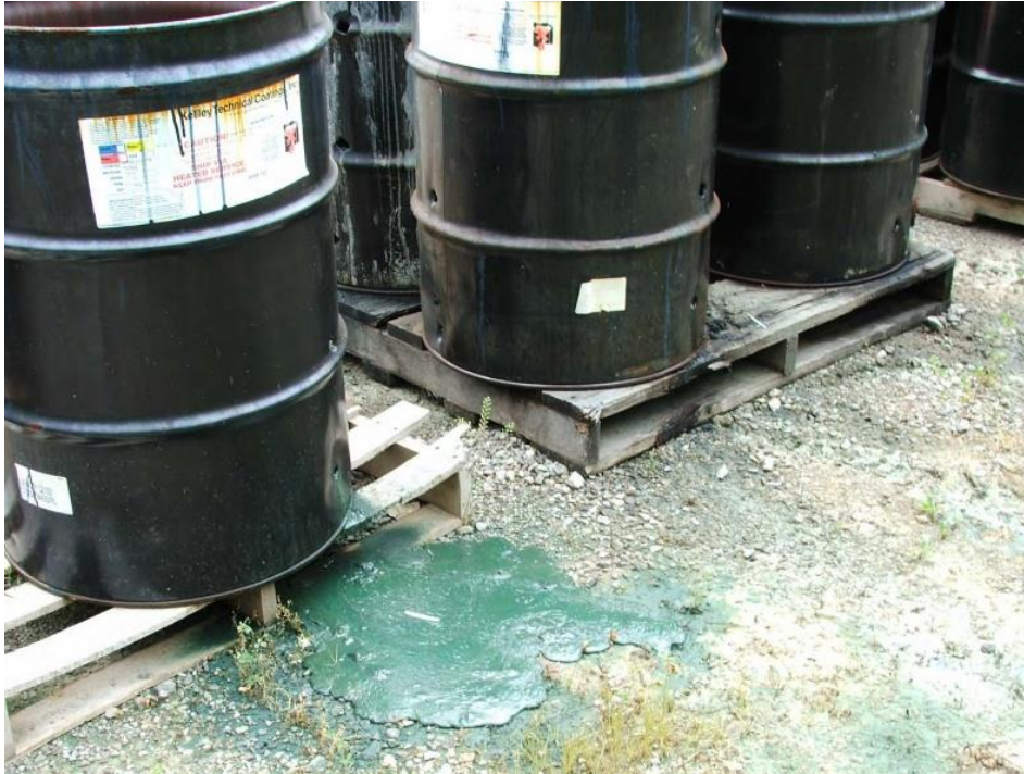
Higher Risk for Stormwater Impact: Drums stored without spill containment
