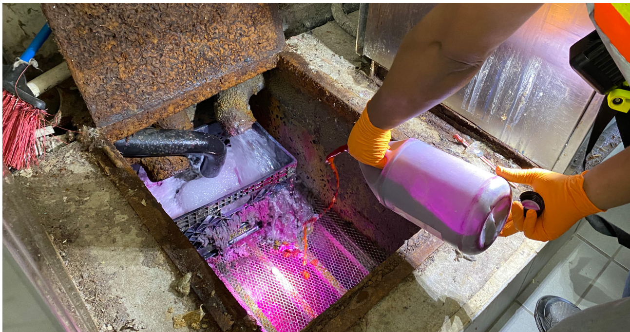
DEP conducts dye test to track down illicit discharge.
