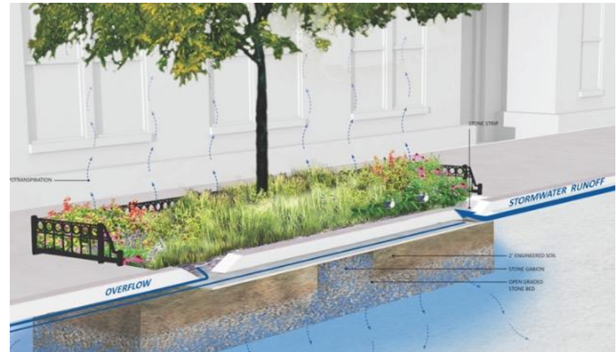
Example rain garden schematic
